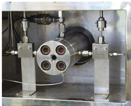
High-pressure vessel designed to withstand pressures of up to 1,000 atmospheres
