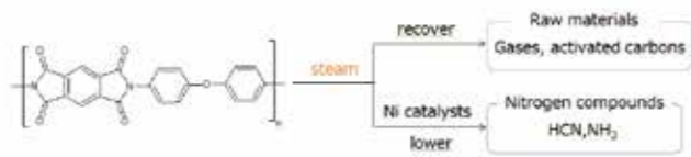
Fig.1 Scheme of steam pyrolysis of polyimide
